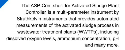
Additionally, by measuring the oxygen uptake rate (OUR) of bacteria in real-time, the ASP-Con can provide indicators of bacterial activity through respirometry.
